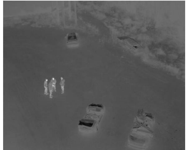
An image taken from the drone using the infrared camera. An example of how the drone can be used in rescue operations to find missing subjects.
